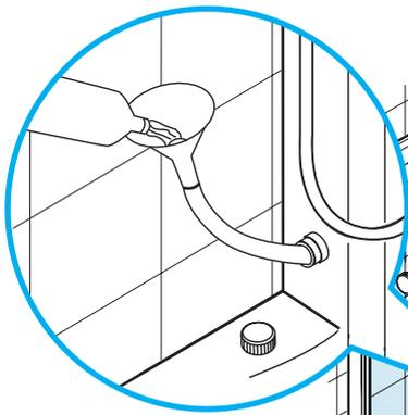
Filling opening on all acrylic and aluminium panels (shown using steam bath Las Vegas as an example)
